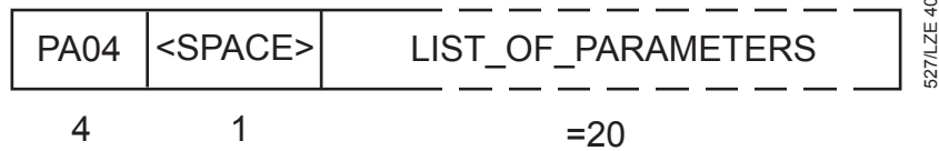
Figure 132 Structure of the PA04-command text field.
